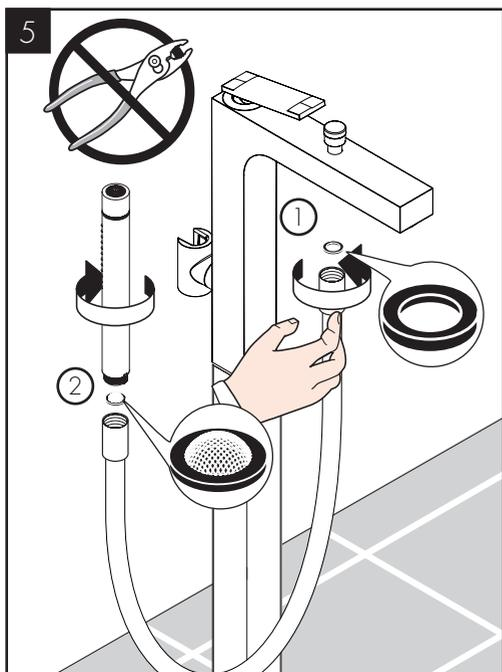
Place the black rubber washer in one end of the hose. Attach this end to the tub filler .
