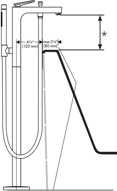
If measurement \* is less than the air gap required in your area, install this item with extension 93882000 (sold separately).
