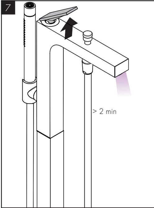
Flush the hot and cold supply lines for at least two minutes.
