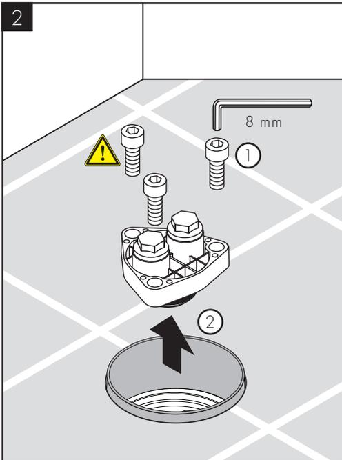
Remove the flush housing screws.
