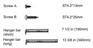
Note: Hanger bar (short) only can slide into channel A.
