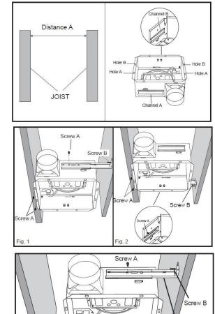
2.Mount with mounting holes and hanger bar Slide one hanger bar into the channel on the housing and adjust to fit between framing. Hold housing in place so that the housing contacts t
